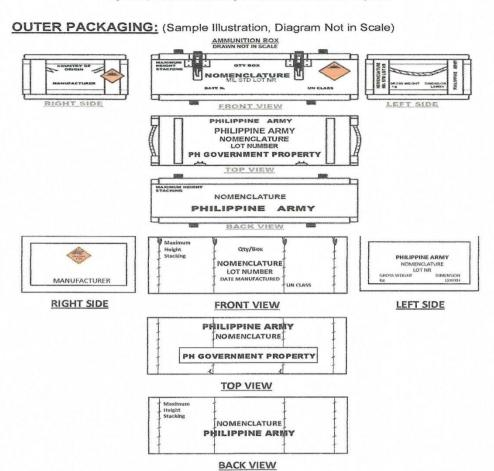
**Note:** The illustrated diagram is just an example purposely to serve as reference. Placement, font size, and font-style are manufacturer's standard. Refer to Technical Specification for the minimum required markings.
