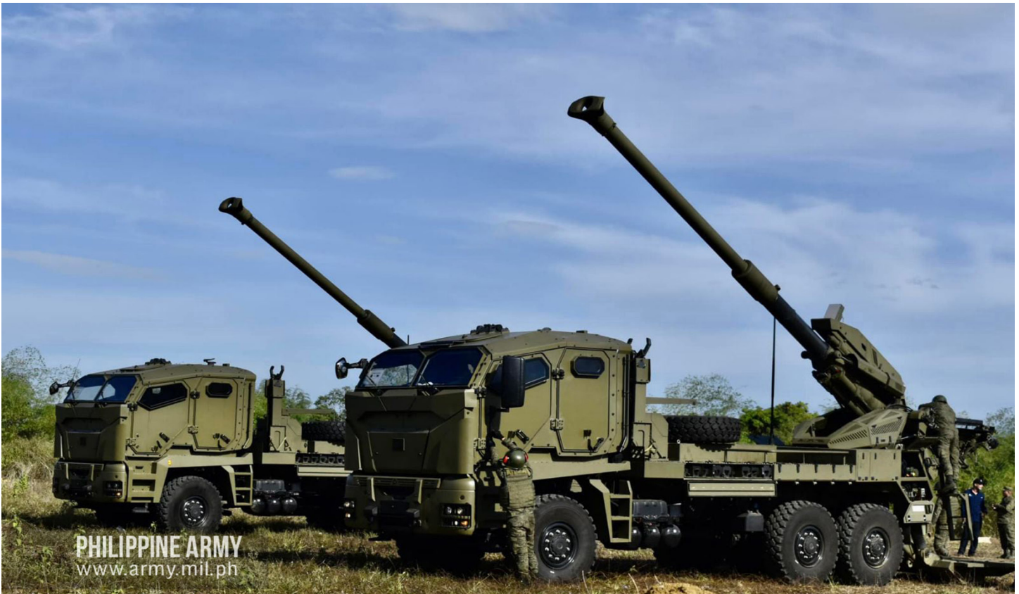
Autonomous Truck Mounted Howitzer System (ATMOS) 155 mm/52 caliber self-propelled artillery pieces at the Fort Magsaysay Military Reservation Area
